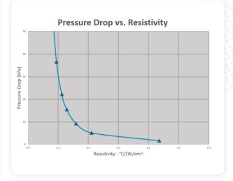
$$R^* = Resistivity \equiv \frac{T_c - T_{in}}{q / A}$$
